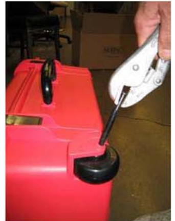
10- REPLACE PIN WITH "7047 Rev B" PIN
