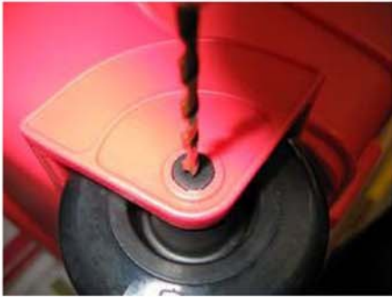
3- INSERT SCREW (#8 X 1 5/8" Phil Self-Drilling Screw)
